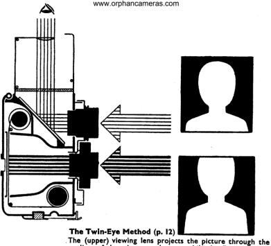
Ine (upper) viewing lens projects the picture through the medium of the mirror to the eye, while the (lower) taking lens guides it to the negative. As the two lenses occupy different positions, the two pictures will cover slightly different areas. To leave a margin for errors the focusing screen of the Rolleiflex has been cut smaller than the actual film area. Only with close-ups can the "parallax"—become serious.
